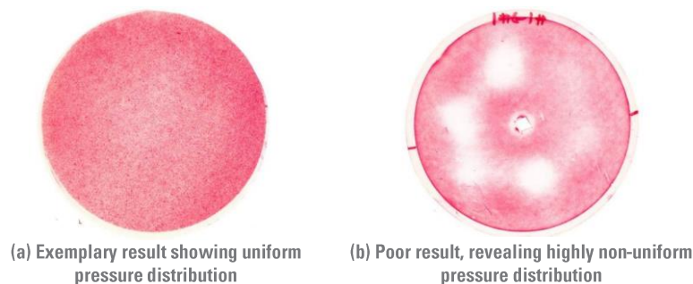
Figure 10. Results from Inspecting the Pressure Distribution using Color-Changing Film
