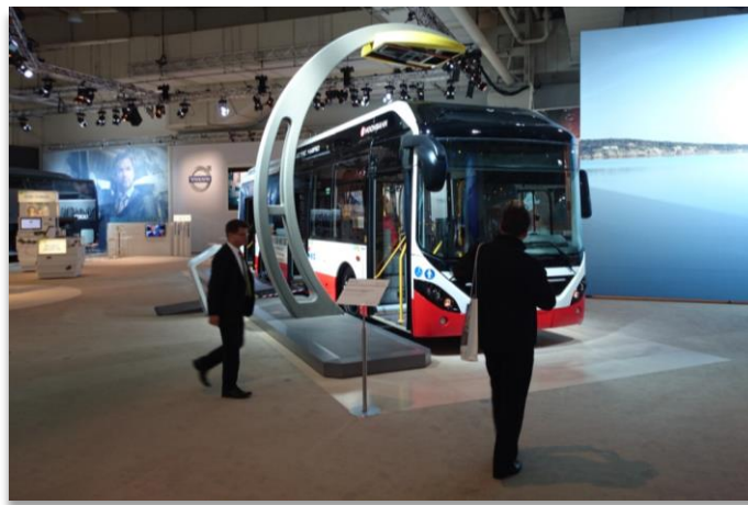
Figure 13. Top-down Pantograph for Opportunity Charging
